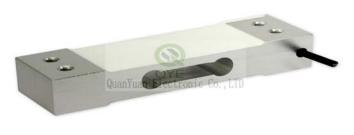
Features: Capacity : 5kg to 120kg High accuracy. Alloy aluminum parallel beam Max. platform size:250x350mm Integral structure,reliable performance,and easy installation
